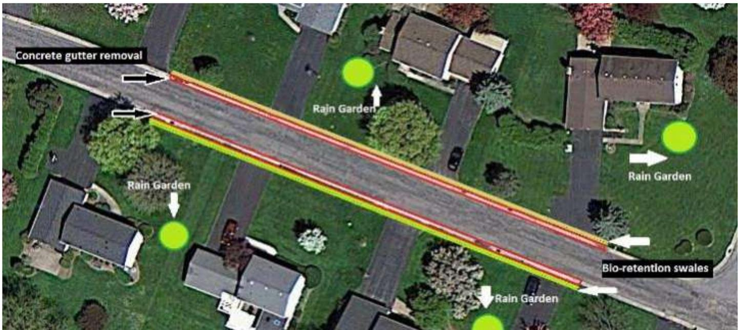
Figure 8: Above is a example of a neighborhood with standard stormwater management practices i.e. concrete gutters along the streets which connect to the stormwater sewer, fair amounts of impervious cover, and roof top connections to the stormwater sewer. Replacing the concrete gutter with bio-retention swales and diverting roof top runoff to rain gardens provide source control and infiltration for stormwater runoff.
