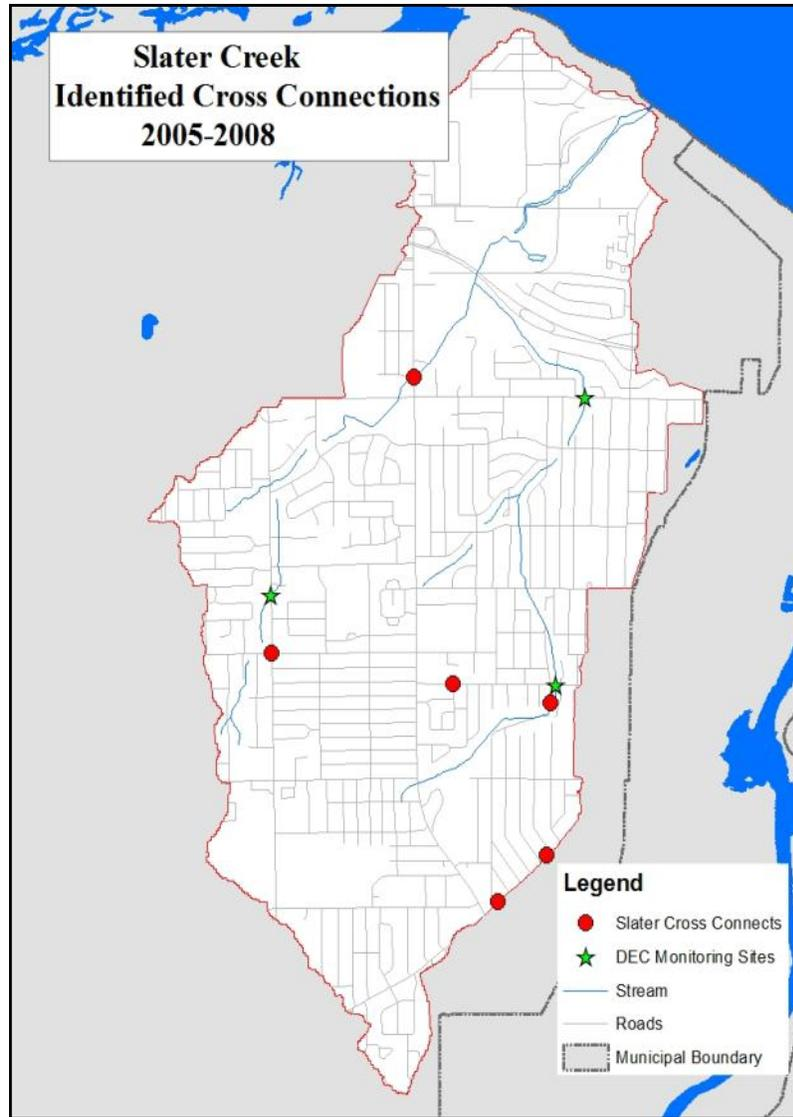
Figure 7 Slater Creek Cross Connections
