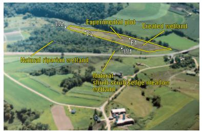
**Figure 1.** Aerial view of the Wisconsin Department of Transportation/U.S. Geological Survey wetland creation site near Wilton, Wisconsin one year after construction. Within the created wetland are experimental plots where design parameters (for example, depth to ground water) were varied. The locations of intensively instrumented sites in the natural and created wetland are also shown.
