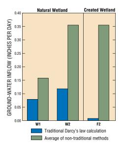
**Figure 2.** The blue bars represent the values of ground-water flow estimated by using traditional Darcy's law calculations. The green bars represent the inflow measured by innovative methods and demonstrate that traditional approaches can significantly underestimate inflow to wetlands.
