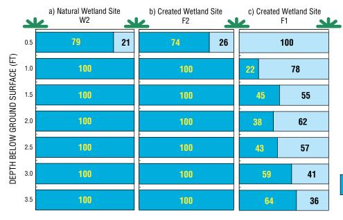
Figure 4. Assessing whether you've created the appropriate hydrology at a created wetland can be difficult. By analyzing the water molecule we can identify the sources of water at different depths in the wetlands. This approach shows that areas of the created wetland have the same ground-water source (a and b). Other areas of the created wetland (c) depend on rain water to maintain water levels and are expected to be drier in times of drought.
