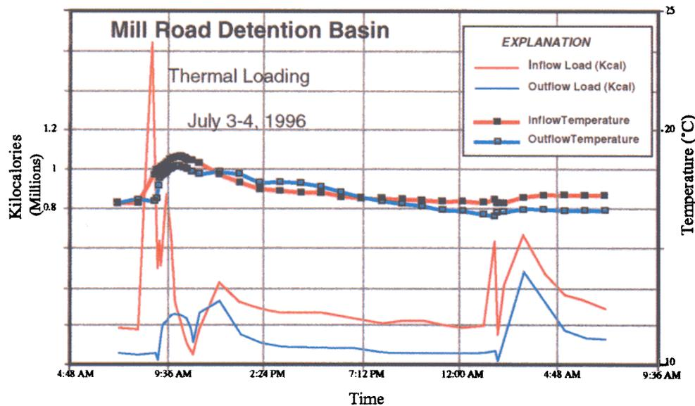
This graph illustrates the relation between inflow and outflow water temperatures and the thermal loads\* computed from temperature and discharge during and after a summer storm at the Mill Road detention basin in Monroe County. Note that:
