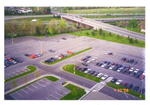
Large areas of our community are covered with impervious surfaces such as roads and parking lots. The stormwater runoff from these areas is a major source of pollutants to our water resources. Wetlands can be created to remove the pollutants from stormwater runoff.
