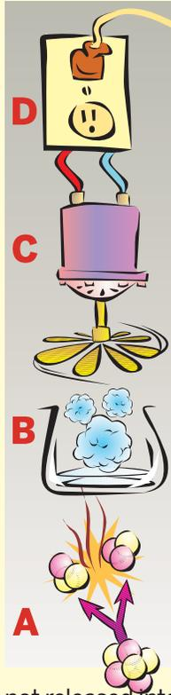
Power plants create electricity by running steam turbines, which are powered either by fossil fuels – coal, oil, natural gas – or by nuclear power. Nuclear technology produces energy by splitting uranium atoms in a process called fission. (A) Fission generates heat that (B) boils water for the steam that runs the (C) turbines, which produce the (D) electricity that we all use – making, for instance, (E) toast for breakfast.
