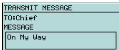
Once you select **SEND**, the message is placed into the *M1501* transmit queue, where it will wait for a few seconds until the *M1501* transmits it to the *SPARKGAP* network. While messages are in queue, a pending transmission icon will appear next to the **VIEW TRANSMITTED MSGS** main menu item. Once the message is successfully transmitted, this icon will vanish.
