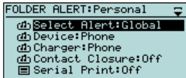
The Folder Setup menu selection sets the alerting behavior of individual message folders, overriding the Global Setup values. Selecting this menu item will present a FOLDER ALERT menu containing one menu selection for each folder. Selecting a particular folder allows you to edit 7 settings for that folder:
