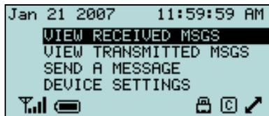
The main menu is the first screen displayed by your *M1501* after power-on. It provides menu options into the four main functions of your pager. You can use the up/down button to select one of the following choices:
