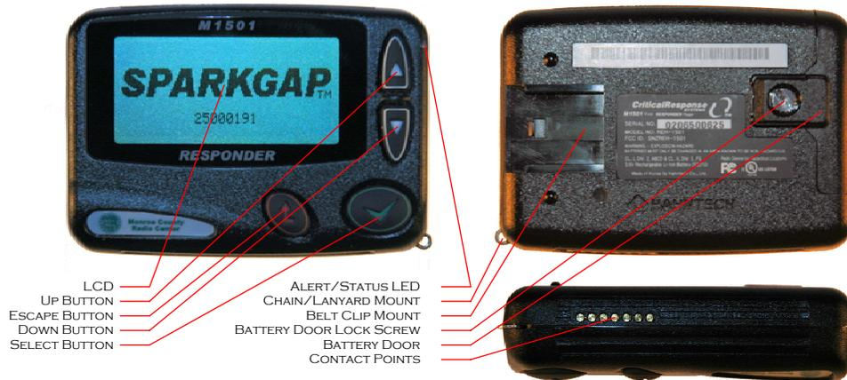
Your *M1501* consists of a digital radio and CPU in a polycarbonate housing, a 160x64 LCD display, four buttons, a replaceable/rechargeable Li-Ion battery pack, and contact points for charging and programming. It also comes with a belt holster and detachable belt clip.
